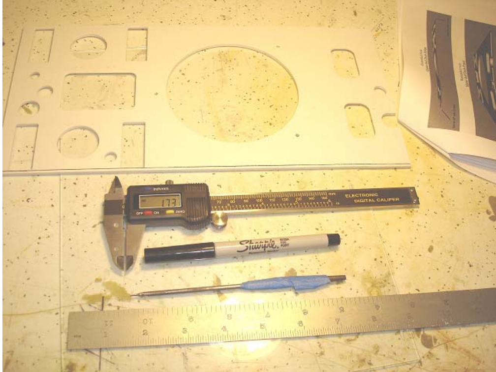
Above are seen from the top, the bottom side of the upper deck with a measurement of 1.73mm drawn on the inside of the lower edge, digital vernier caliper, permanent marker, metal scribe, steel ruler, and off to the right the angle guide provided by WeCoHe.
